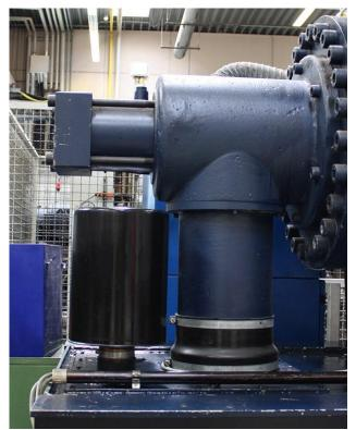
Figure 7: Breather filter on pedestal
