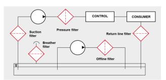
Figure 3: Diagram of filter types
