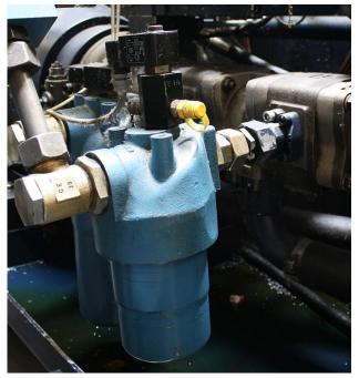
Figure 4: Pressure filter with differential pressure sensor
