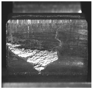
Figure 8: Tooth flank damage
