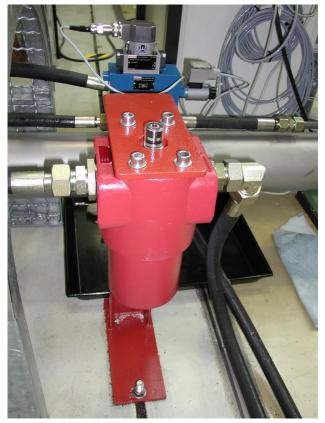
Figure 1: Filter on a hydraulic power unit
